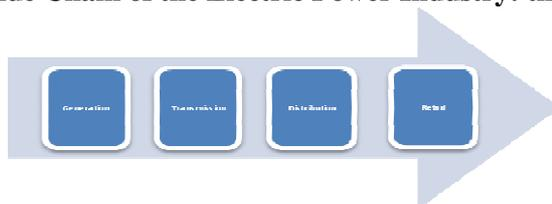
The electricity value chain has four stages: generation from a variety of sources; transmission which is the transport of high voltage electricity over long distances; distribution as the local transportation at lower voltage to final customers; and at last, the retailing activities which comprehend the selling and billing to final consumers..
